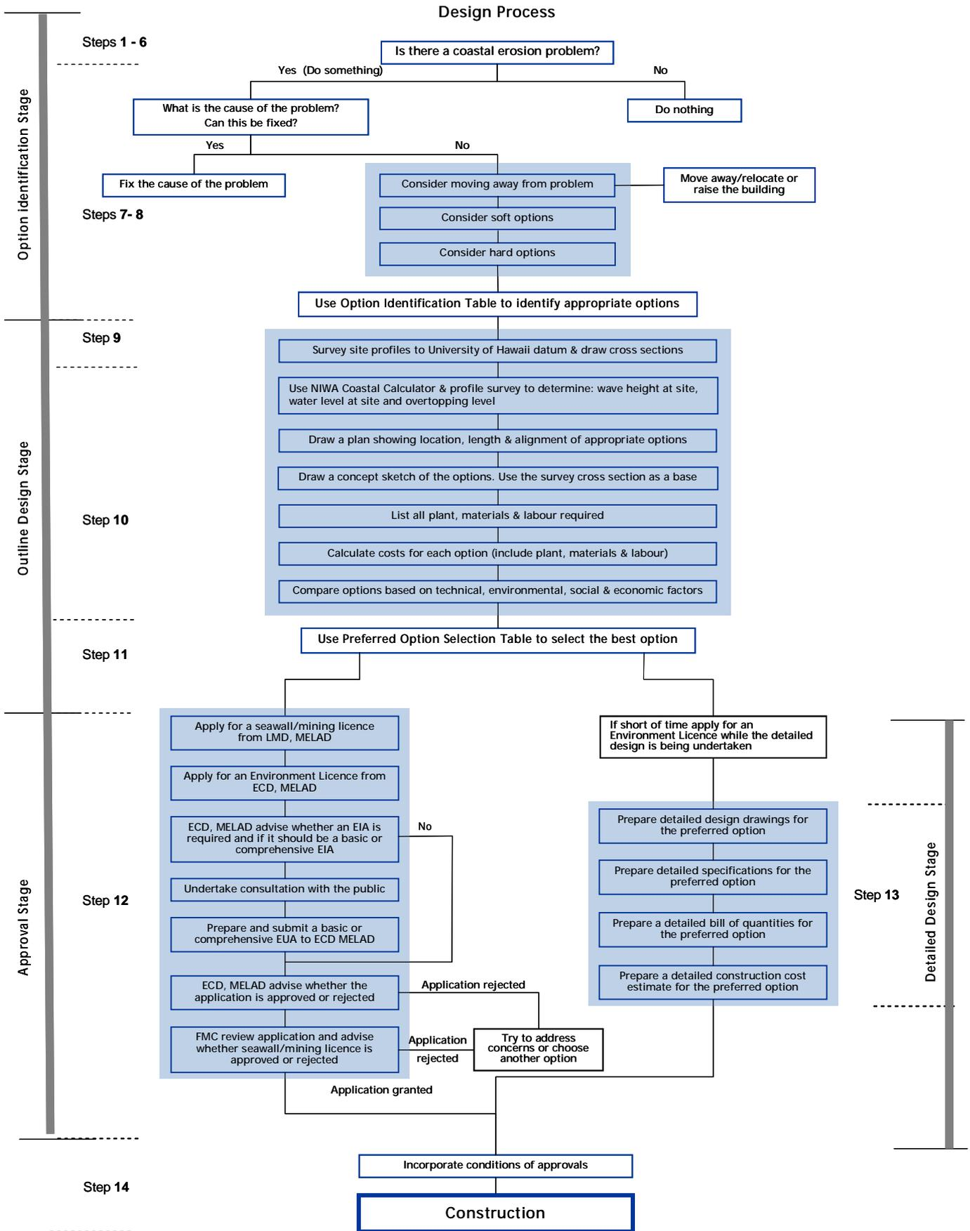
Figure 2 – Design Process Flowchart
