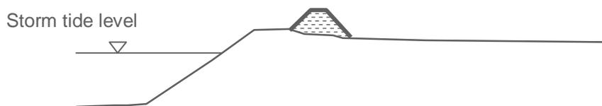
**Figure 6 – Typical Earth Embankment (diagrammatic)**
